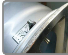
1. Install valve stem into the valve hole of the wheel.
