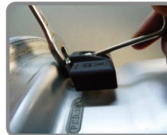
5. Install sensor, make TPMS sensor adjusted to fit the drop well of the wheel. Use wrench to hold valve stem and maintain vertical position, then tighten screw with 4Nm (±0.5) torque.
